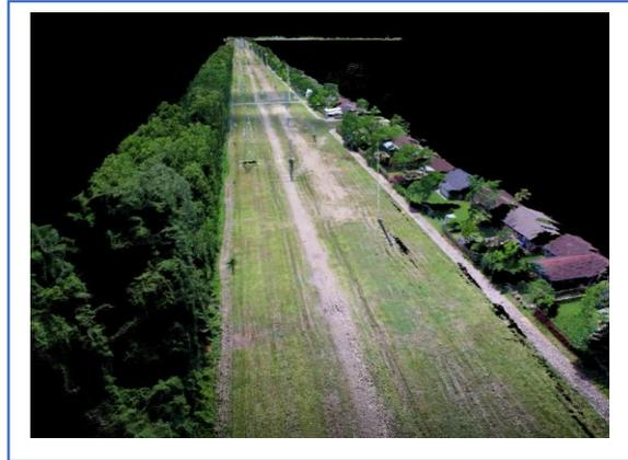
Fig. 6. 3D Point Cloud of Pipeline Right-of-Way, 80 Percent Overlap
