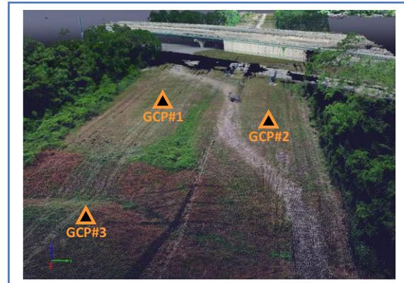
Fig. 1. 3D Point Cloud with Minimum GCP Profile
