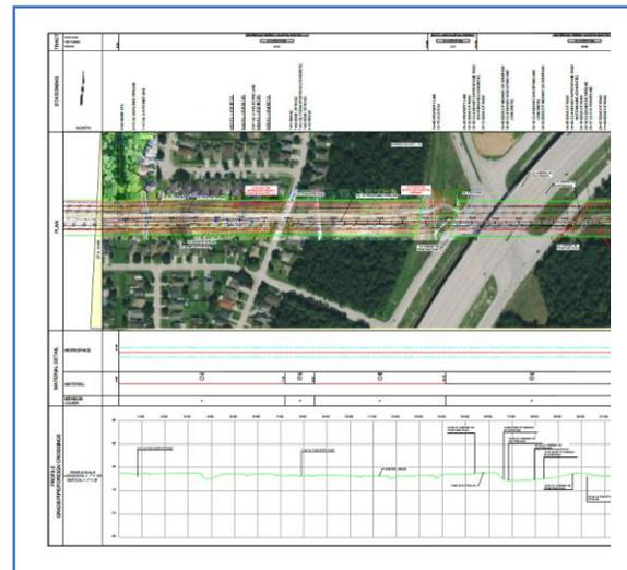
Fig. 8. Alignment Sheet Produced from UAV Aerial Photogrammetry
