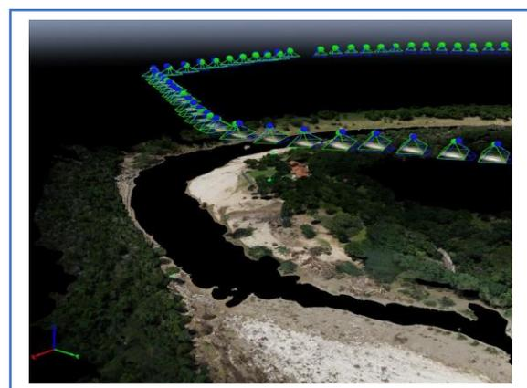
Fig. 5. Flight Path with Semi-Autonomous Operator Control
